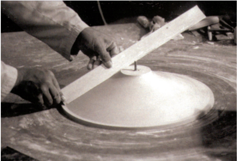
Figure 2: One-sheet hyperboloid crafted with a ruler (from: Burry 2007).
